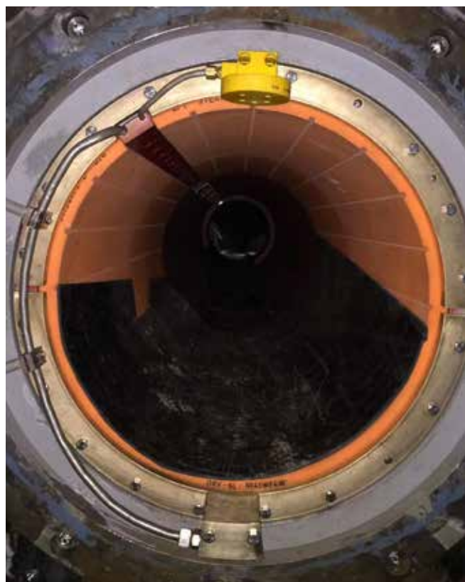
Thordon's COMPAC propeller shaft bearing installed with the Bearing Condition Monitoring System
