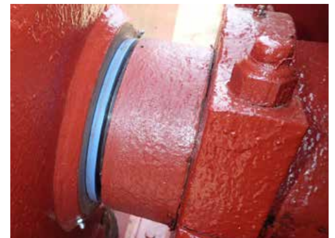
Thordon's ThorPlas-Blue retrofitted to winches aboard a tanker
