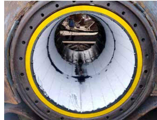
The Thordon Composite bearing being freeze fit into the cutterhead shaft.
