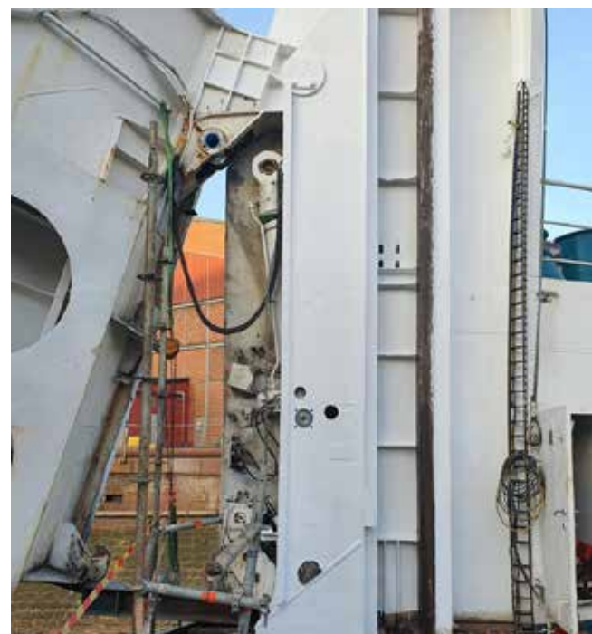
ForSea Ferries has provided Thordon with its first reference for ThorPlas-Blue bushings to the bow doors of a ro-ro ferry
