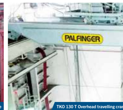
TKO 130 T OVERHEAD TRAVELLING CRANE - For handling of 130 t thrusters - Fully electric
